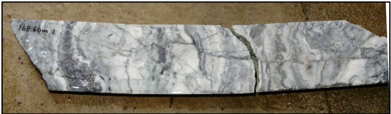
FIGURE 7-16 BANDED LOW SULPHIDATION EPITHERMAL QUARTZ VEIN FROM DRILL HOLE RD10-009 (168.60 M). EXAMPLE OF PRESERVED PRIMARY TEXTURES
